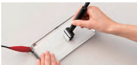
Marking a metal surface using a GOCCOPRO 100-exposed screen.
